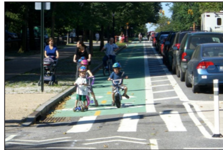
Two-way parking protected bike path on a one-way street, Prospect Park West, Brooklyn
