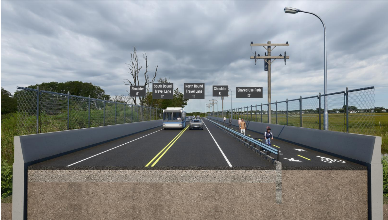
Alternative 2 Rendered Cross Section View
