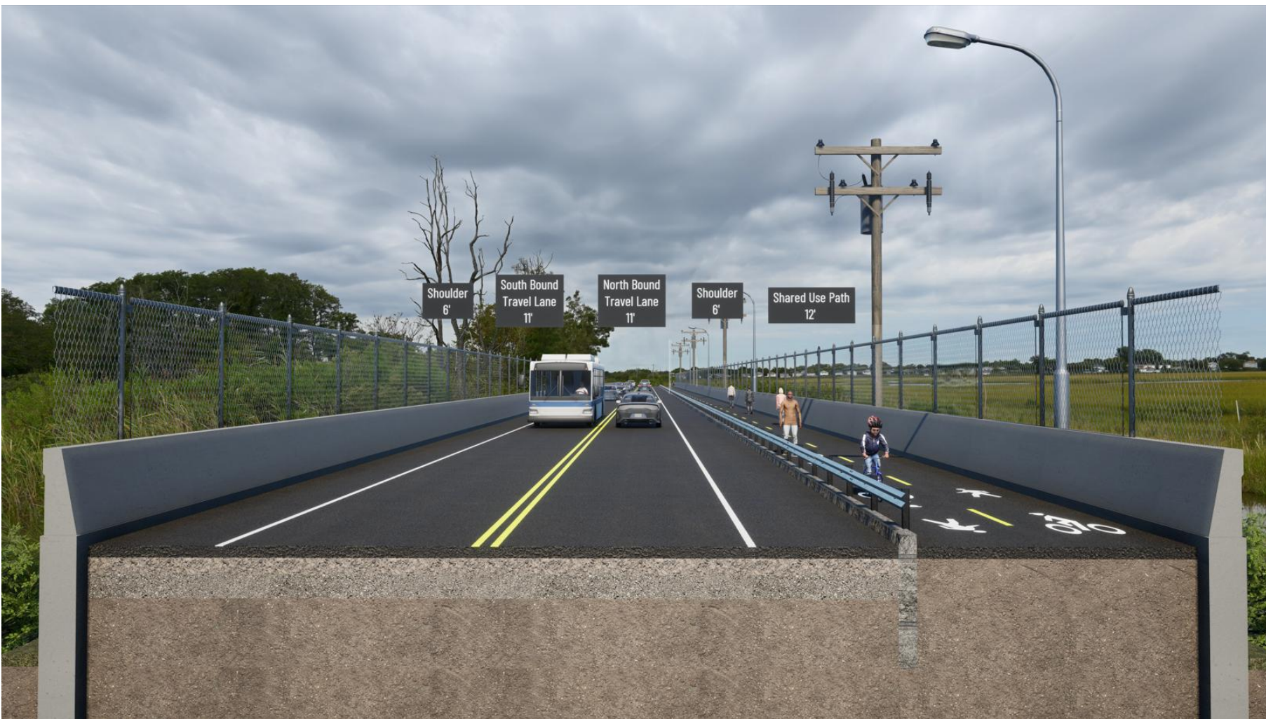
Alternative 1C Rendered Cross Section View
