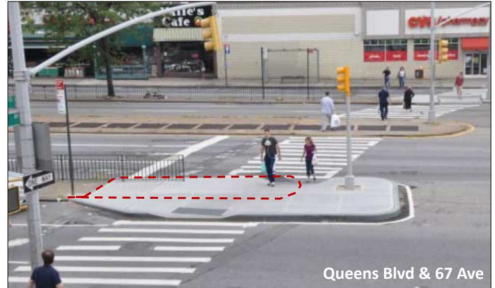
Median tip extension/widening
