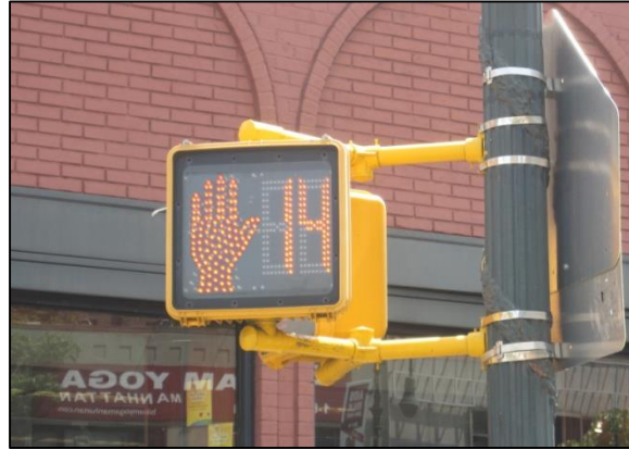
Countdown signals: tell pedestrians how much more time they have to cross
