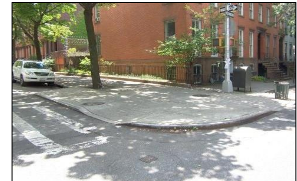
Sidewalk extension: shortens crossing distance, slows turning cars
