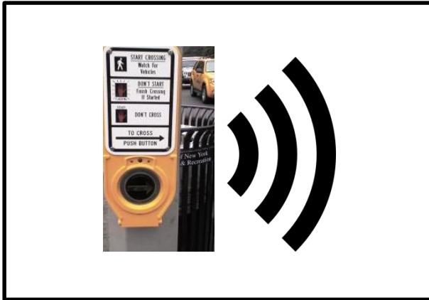
Accessible Pedestrian Signals (APS): provide audible signal in areas with persons with vision impairments
